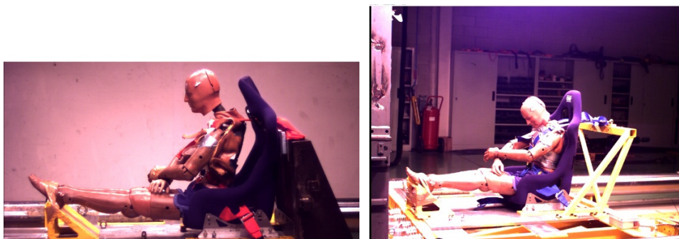
Figure 6: Instant pictures of the dummy during impact.
