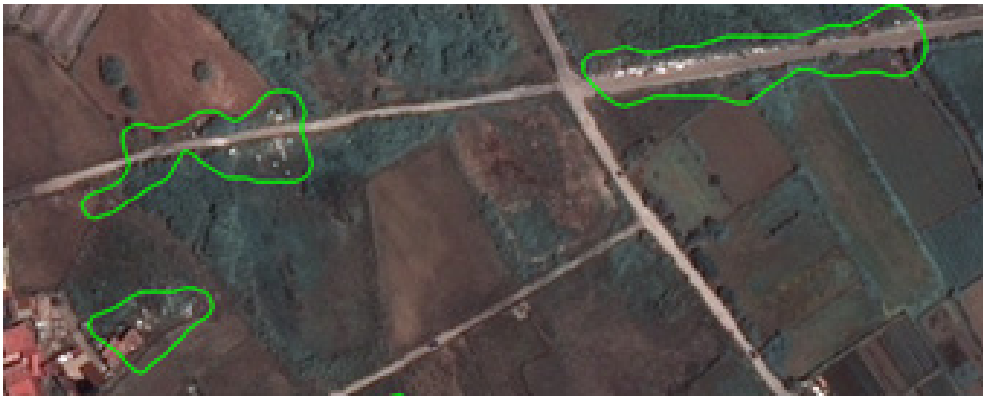
Figure 1: Micro-dumps automatically detected in VHR satellite imagery by means of a target detector based on scattering transform [4].
