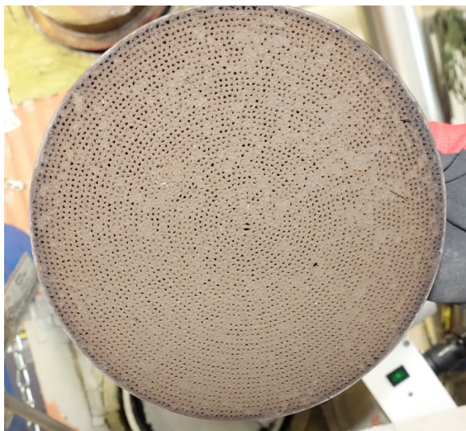
Figure 7: Clogged catalyst by particulate matter after four test days of Stove 2.
