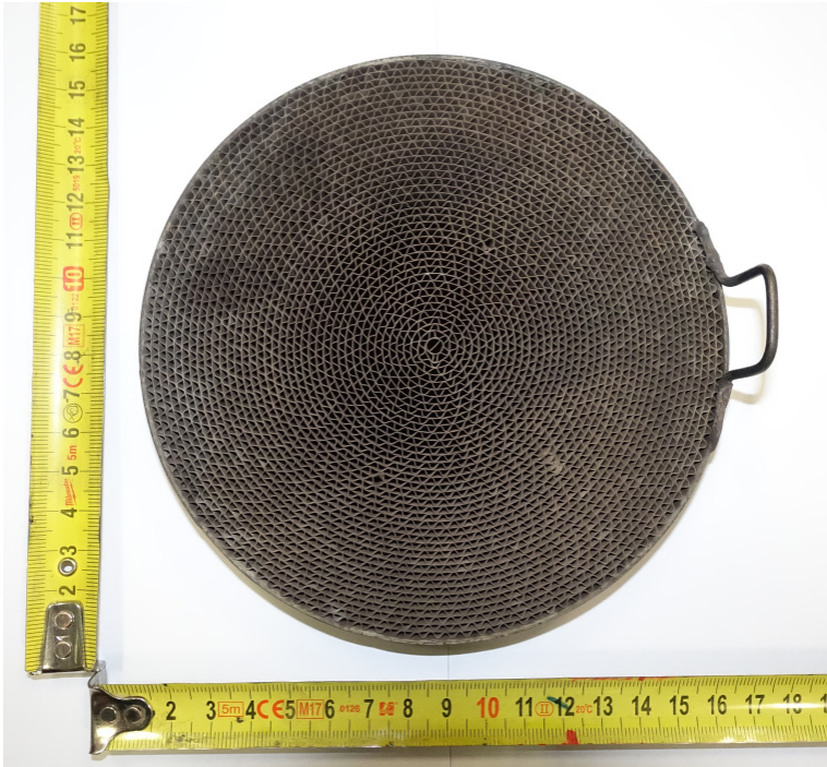
Figure 1: Honeycomb catalyst before combustion tests.
