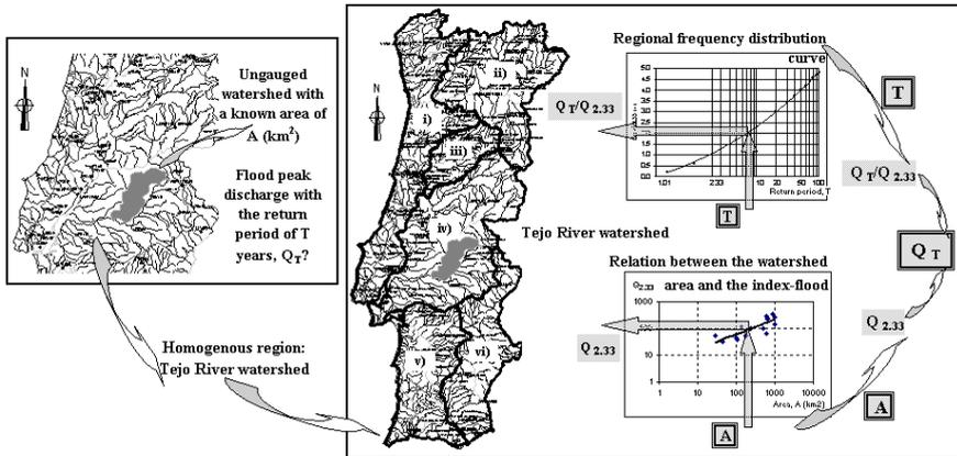
Figure 9: Index-flood method. Evaluation of flood quantiles based on the values of the watershed area and the return period. Schematic steps.
