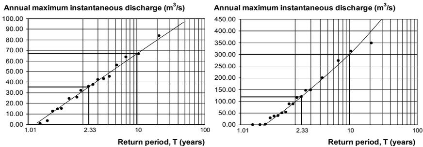
Figure 3: Local frequency distribution curves at Pai Diz (left) and Monforte (right) stream gauging stations.
