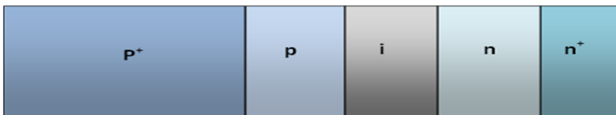
Figure 1: Scheme of GaAs p^+ - pin - n^+ structure.
