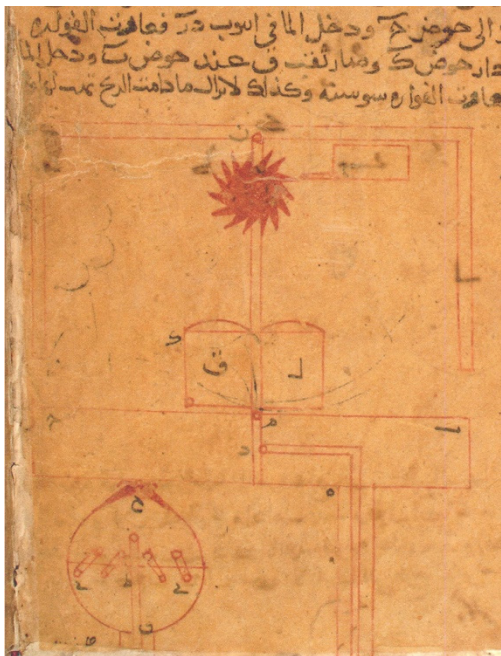
Figure 2: Banū Mūsā, fountain operating by wind or water (folio 37 verso, Arabus 317, Vatican Library). On the right is a scheme of the function of the device.
