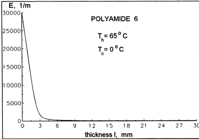
Figure 5: Dependence of extinction coefficient  $E(l)$  on polyamide 6 sample's thickness and under condition  $\Delta T = 65 \text{ K}$
