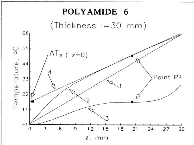
Figure 6: Calculated temperature distribution in the polyamide 6 sample. 1-pure conduction, 2-radiation-conduction, 3-first derivative of curve 2 at point ( $z=0$ ), 4-extrapolation of linear section of curve 2.
