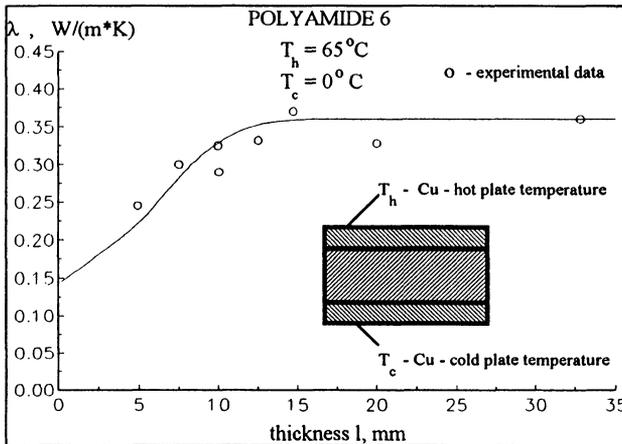
Figure 3: Approximation of polyamide 6 thermal conductivity experimental data vs. a specimen thickness  $l$  and a schematic diagram of physical system ( $\Delta T = T_h - T_c = 65\text{K}$ ).
