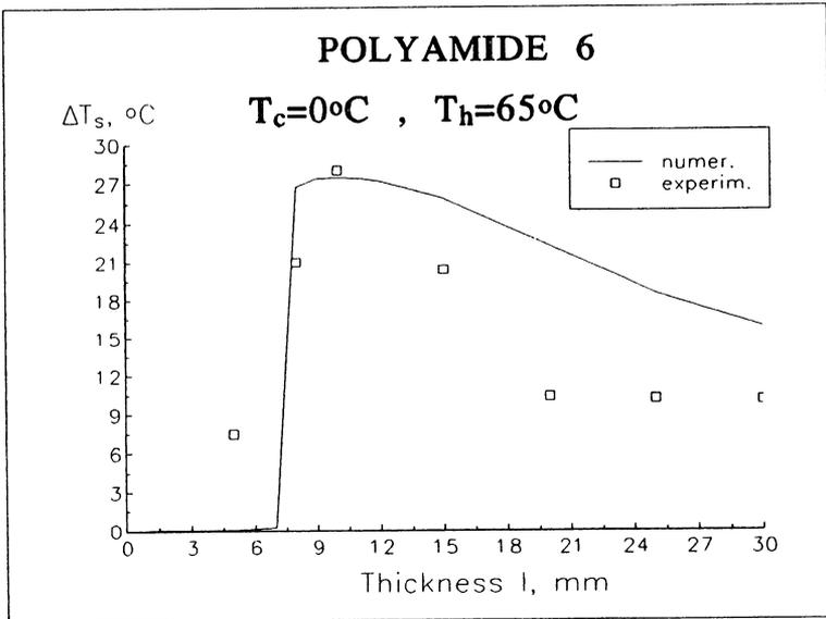
Figure 7: Calculated and experimentally measured temperature slip  $\Delta T_s$  for polyamide 6 sample.
