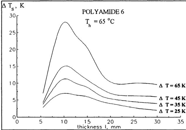
Figure 2: Dependence of the measured temperature slip  $\Delta T_s$  near the cooler for the polyamide 6 sample on its thickness  $l$  for various temperature difference values  $\Delta T$  between the heater  $T_h$  and the cooler  $T_c$ .
