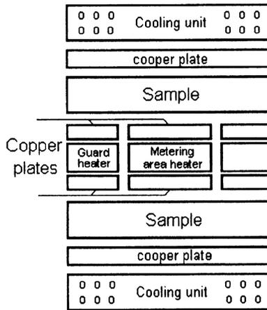
Figure 1: Measurement pile of a guarded hot plate apparatus for studies of thermal conductivity of plastic.
