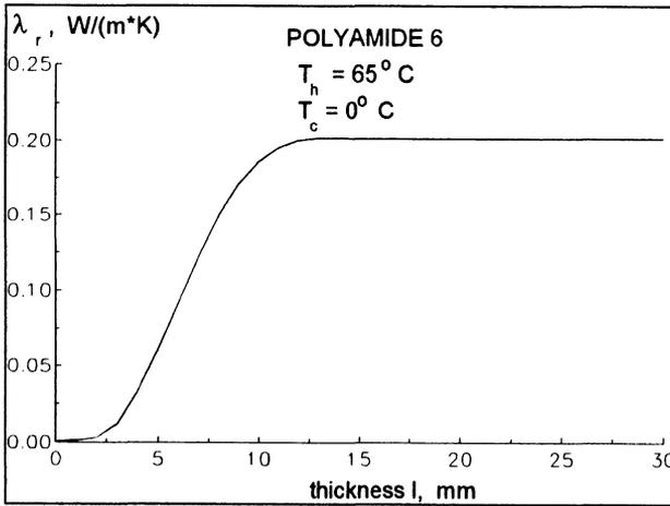
Figure 4: Dependence of radiative thermal conductivity  $\lambda_r$  on sample's thickness  $l$  under constant temperature difference  $\Delta T = 65$  K for polyamide 6.
