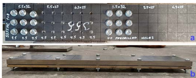
Figure 2: Example of (a) test specimen with screws drilled in; and (b) drillability test assembly pair of plates (4 + 8 mm plates with 1 mm gap).
