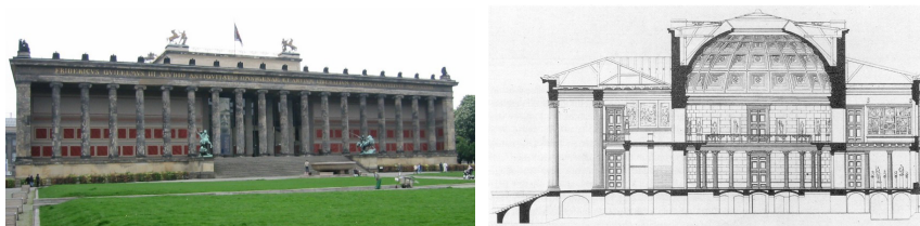
Figure 1: Left: Altes Museum, view from the Lustgarten. Right: Cross section of the Altes Museum showing the different construction elements in the entrance hall, in the rotunda and in the cellar.
