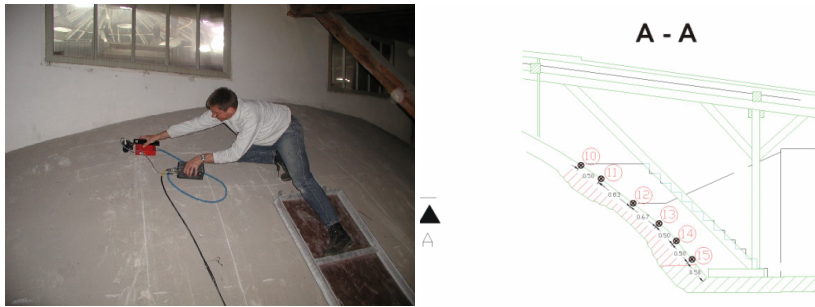
Figure 6: Left: Photo of the radar measurements at the cupola of the rotunda. Right: Cross section with radar traces of one part of the cupola.
