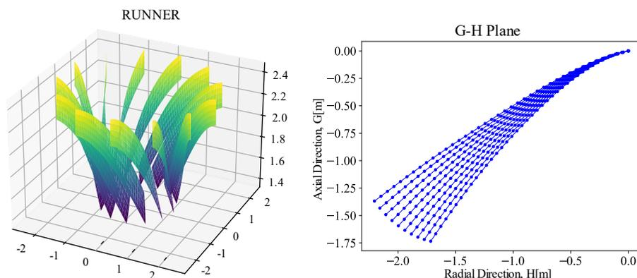
Figure 4: Design of a blade arrangement proposed by the developed Python code and runner blade radial view.
