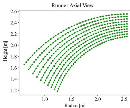
Figure 5: Runner blade axial view.
