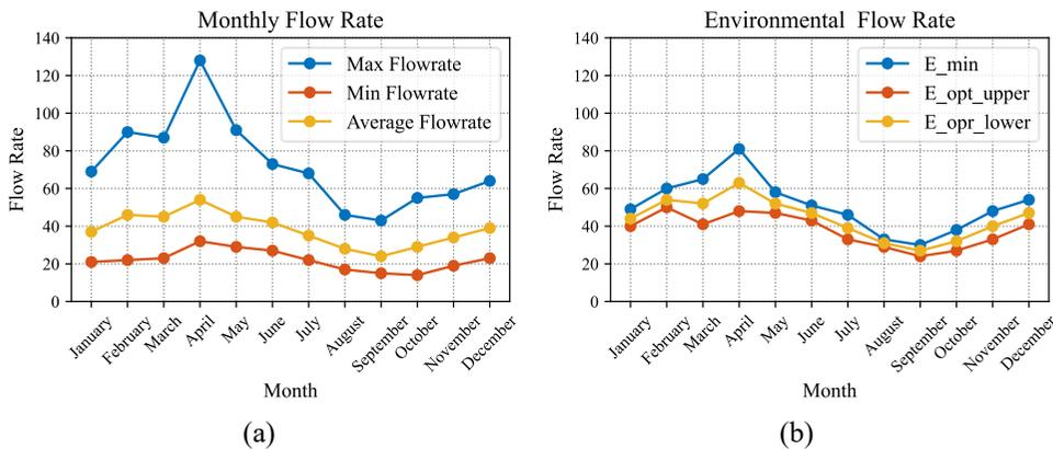
Figure 3: (a) Monthly flow; and (b) Environmental flow rate obtained from hydrological station H148.
