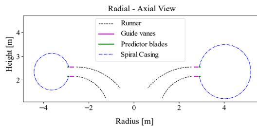
Figure 7: Spiral casing and runner radial axial view.
