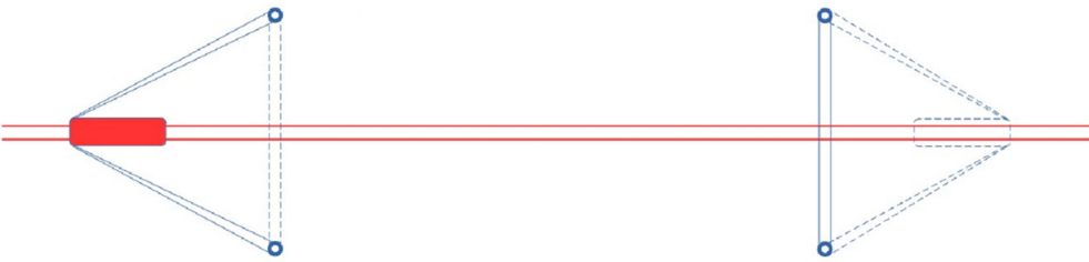
Figure 13: Rubber belt drive. Start = full lines; Stop = dashed lines.
