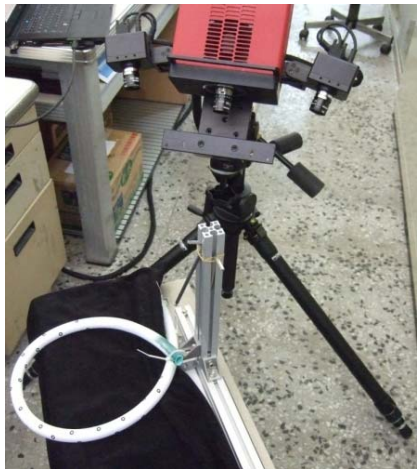
Figure 13: 3D measurement for verification by using Atos system.
