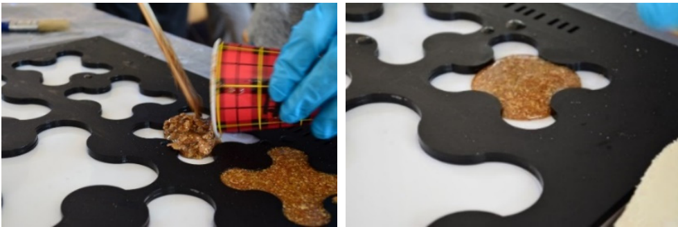
Figure 6: Two units' sizes during casting process in the mould.
