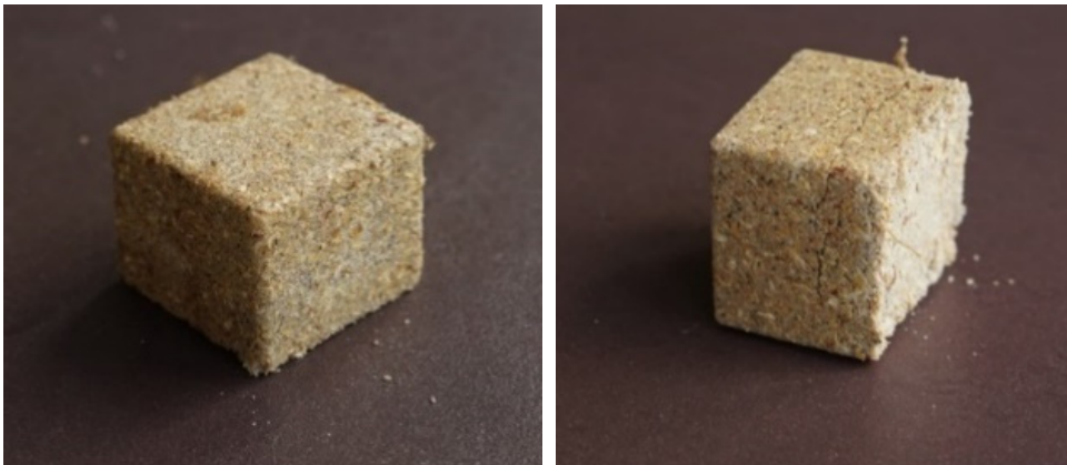
Figure 8: Two samples after heating using corn starch with fine and coarse shells.
