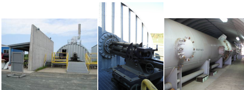
Figure 4: Muffler installation to collect air samples at the muzzle of the gun in a confined area.
