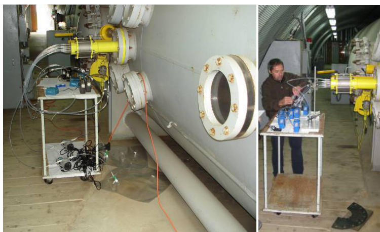
Figure 5: Sampling station at the Muffler installation.
