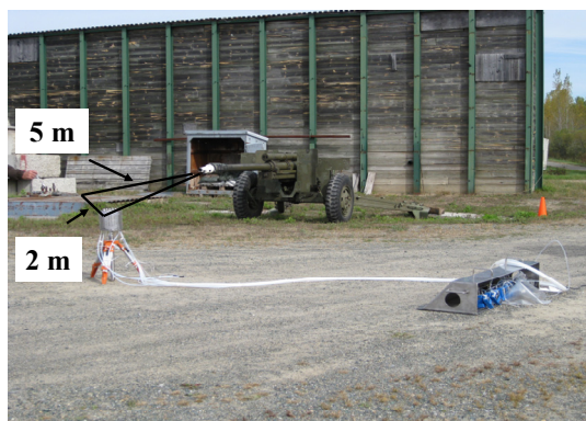
Figure 3: Outdoor set-up for air emissions sampling at the muzzle of the 105-mm gun.
