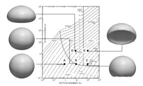
Figure 4: Bubble diagram of Grace for the shape and terminal velocities of gas bubbles in quiescent viscous liquids, reproduced from Clift and Weber [7]. The simulated cases are indicated with capitals.
