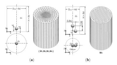
Figure 2: The schematic diagram of the solution domain and mesh configuration. (a) Single bubble rise: The mesh is densified around the symmetry axis of the cylinder  $(M_1:7.6\times10^5cv\equiv15cv/d,\,M_2:1.4\times10^6cv\equiv20cv/d,\,M_3:2.3\times10^6cv\equiv25cv/d,\,M_4:3.4\times10^6cv\equiv30cv/d)$ . (b) Bubble merge: The mesh is uniformly distributed in the cylinder  $(M_5:1.4\times10^6cv\equiv25cv/d)$ .
