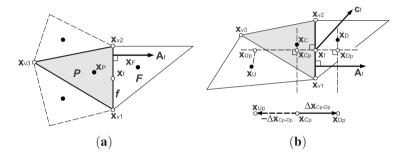
Figure 1: Nomenclature used in spatial discretization: (a) Source term and diffusive node stencil. (b) Convective and compressive node stencil.
