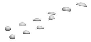
Figure 5: Oblique bubble coalescence of two initially spherical bubbles. Here  $M=0.0002, Eo=16, \rho_1/\rho_2=100, \mu_1/\mu_2=100.$
