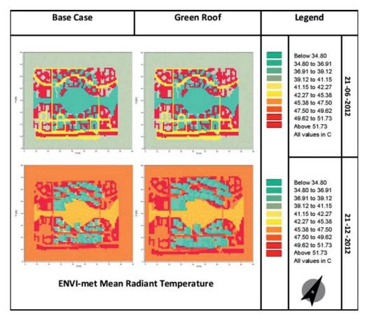
Figure 6: ENVI-met Mean Radiant Temperature (MRT) results of base and green roof.
