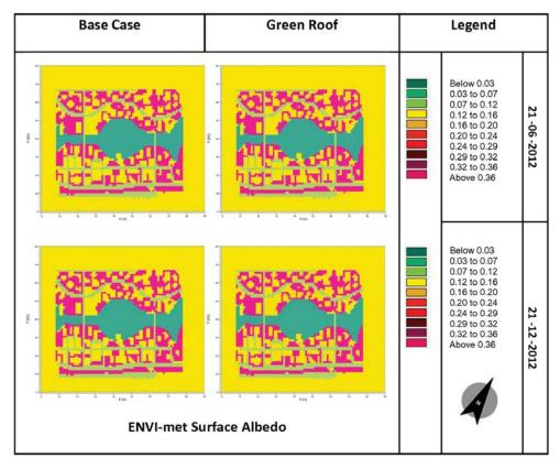
Figure 5: ENVI-met Surface Albedo (SA) results of base and green roof.
