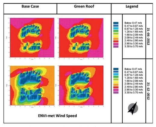
Figure 9: ENVI-met Wind Speed results of base and green roof.
