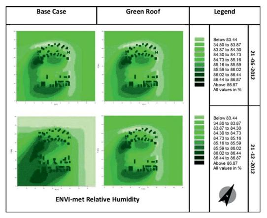
Figure 7: ENVI-met Relative Humidity (RH) results of base and green roof.
