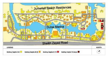
Figure 3: Site Area and Density Diagram.
